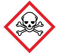
Skull & crossbones (can cause death or toxicity with short exposure to small amounts)
