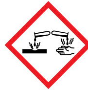
Corrosion (for corrosive damage to metals as well as skin,
